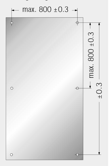
Countersunk holes for countersunk single-point fixings
